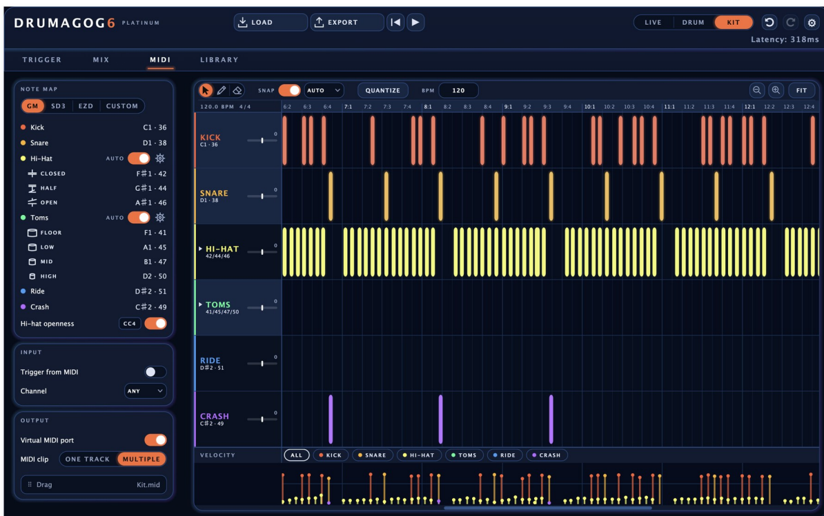
Figure 22. The MIDI page in Kit mode. On the left are the note map and the INPUT and OUTPUT sections. The piano roll on the right shows every hit as a note, with a row for each drum.
