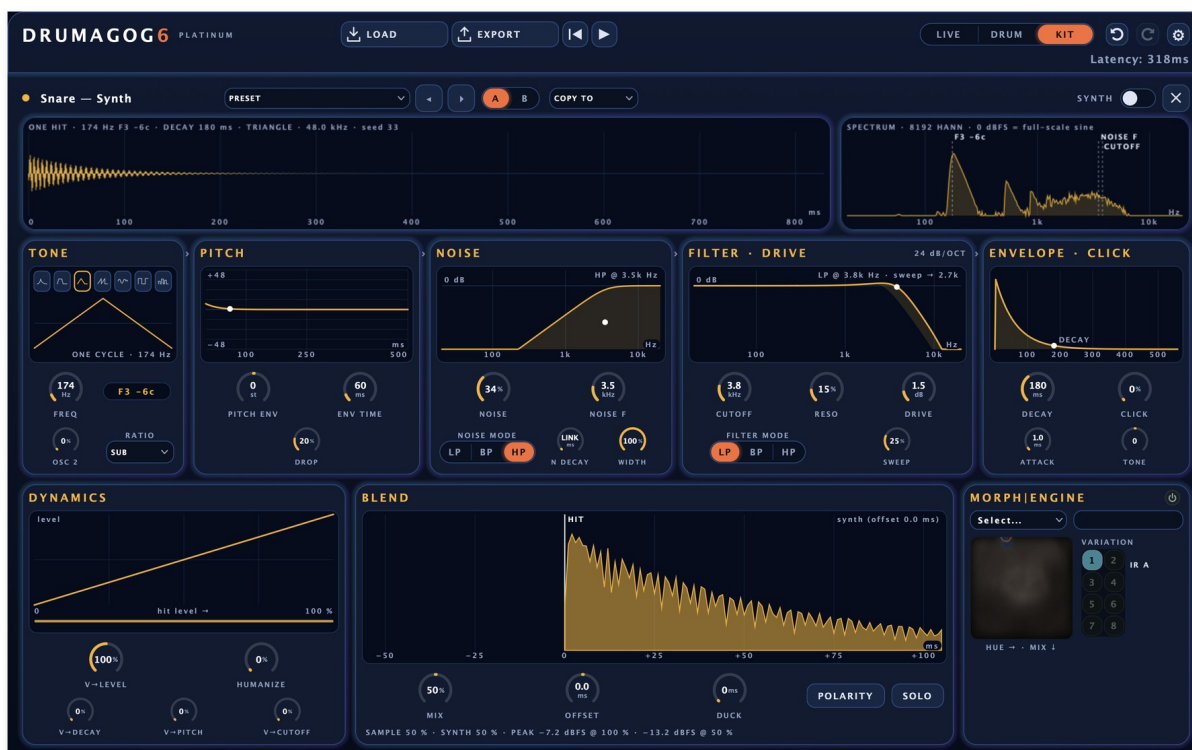
Figure 19. The synth editor for the snare. The displays along the top show one synth hit and its spectrum.
