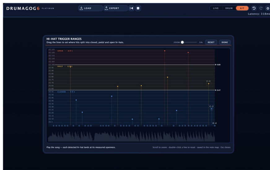
Figure 26. The HI-HAT TRIGGER RANGES window. Each dot is a hi-hat hit. The more open the hit was, the higher its dot sits.
