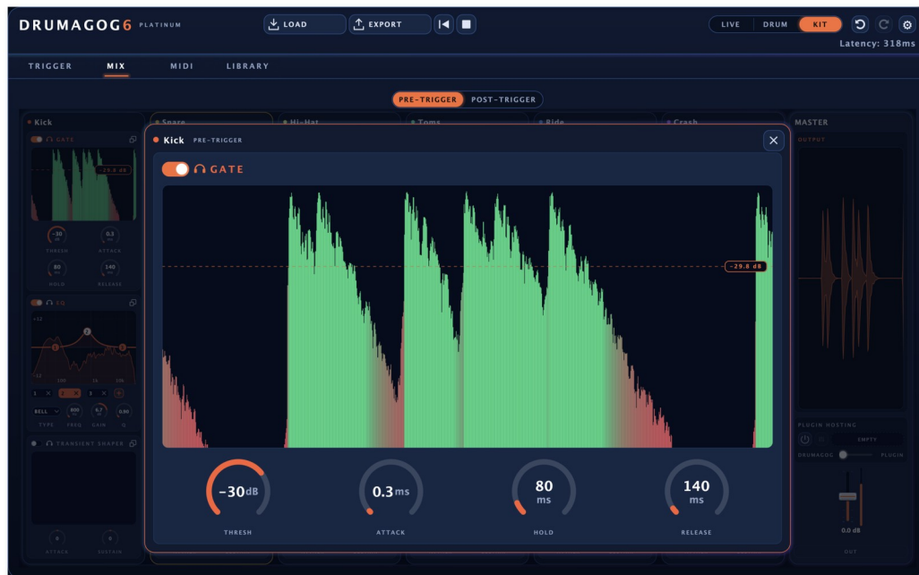
Figure 17. The kick's gate opened in a larger window. In it, what the gate lets through is green and what it cuts is red. The dashed line marks the threshold.
